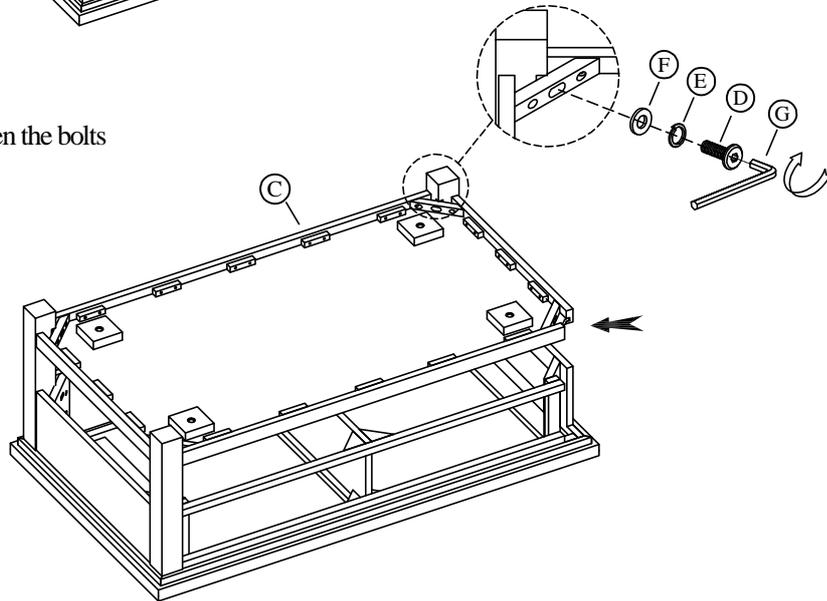
STEP 4: Using the Allen key (G) tighten all bolts
