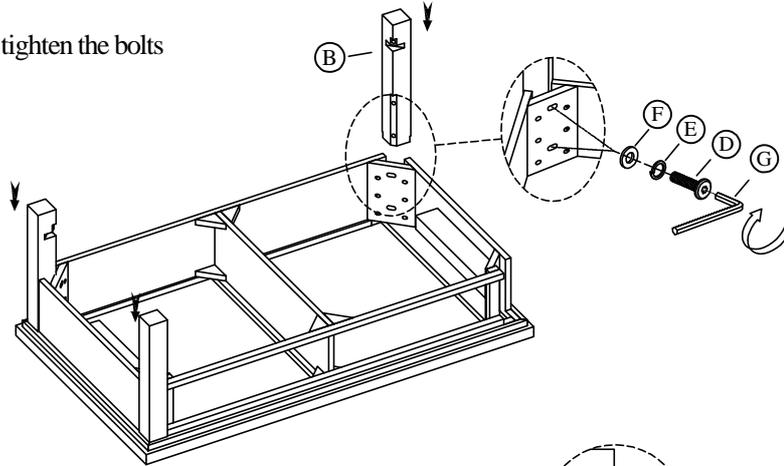
STEP 3: Do not fully tighten the bolts
